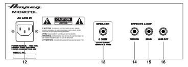
12. AC POWER INPUT: The amplifier is equipped with a detachable power cable that plugs into this IEC Mains socket on the back of the amplifier. The AC power cord should only be plugged into a grounded power outlet that meets all applicable electrical codes and is compatible with the voltage, power, and frequency requirements stated on the rear panel of the amplifier.
