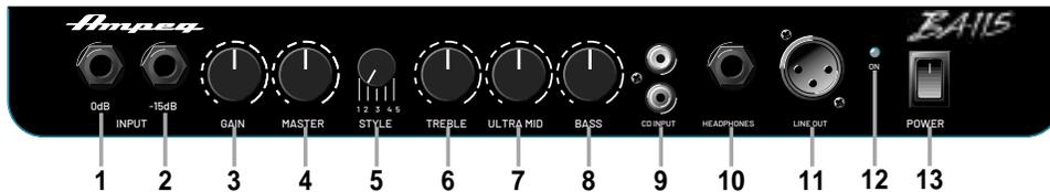
**1. 0dB INPUT:** Connect your “passive” bass guitar here using a shielded instrument cable. This input is not padded and is best suited for basses without active electronics or “hot” pickups.
