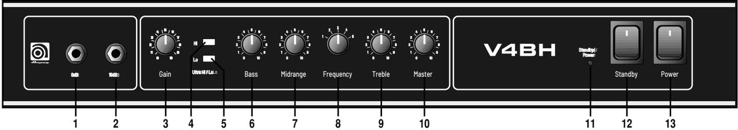
**1. 0dB INPUT:** The signal output from an instrument (active or passive – typically passive) or a line level signal may be connected here by means of a shielded instrument cable. The signal at this jack is sent into the preamp at full strength.
