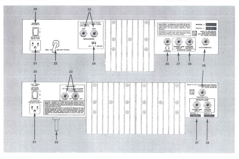
load impedance, considering both jacks, must be at least 4 ohms. The standard internal speaker, normally connected to Int Speaker, is 8 ohms. An additional 8 ohm speaker may be connected to Ext Speaker, which would be a total load of 4 ohms. If your unit is a "head," without a speaker, you may connect up to two 8 ohm cabinets, one 4 ohm cabinet, or four 16
