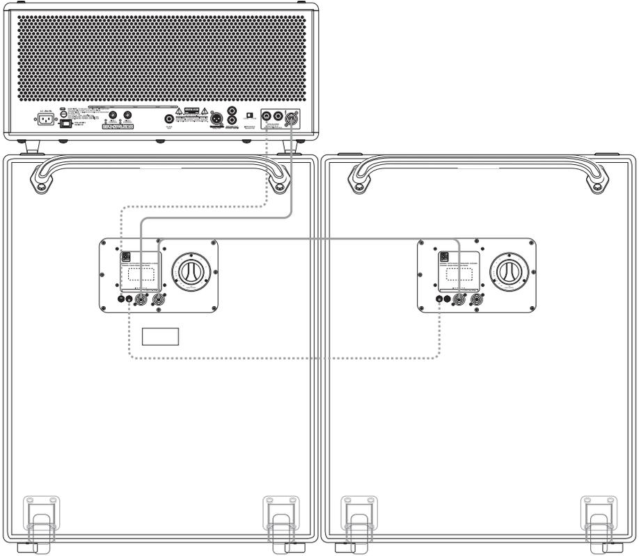
Example 2 above is not as common, but is great for daisy-chaining multiple cabinets. You may connect a speaker cable with 1/4" or Speakon ends from one speaker output of the amplifier to the speaker input of the Ampeg SVT-410HE cabinet. An additional cabinet may be connected by attaching another speaker cable from an open jack (thru) to the input jack of the next cabinet. Multiple cabinets may be daisy chained this way.
