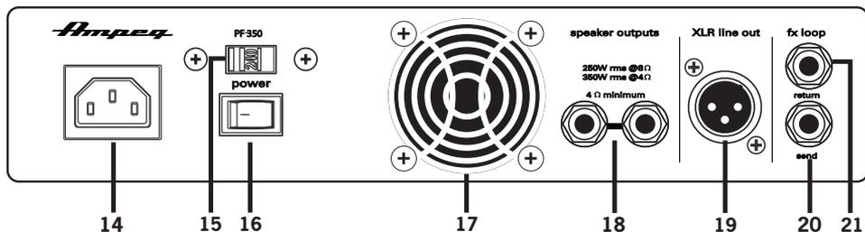
**18. SPEAKER OUTPUTS:** These 1/4" TS Speaker Output jacks supply speaker-level power to the speaker cabinet. The rated power output is 250 Watts RMS into 8 Ω, or 350 Watts RMS into 4 Ω.
