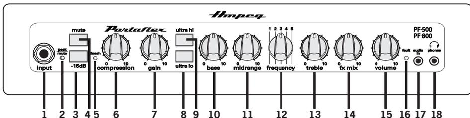
1. **INPUT:** The signal output from an instrument (active or passive) may be connected to this 1/4" Input by means of a shielded instrument cable.
