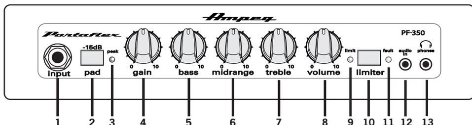
1. **INPUT:** The signal output from an instrument (active or passive) may be connected to this 1/4" Input by means of a shielded instrument cable.
