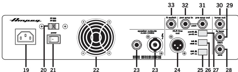
**25. GROUND / LIFT:** Press this switch in to engage the Ground Lift, if necessary, to help eliminate hum at the XLR jack.
