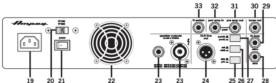
**19. IEC POWER INPUT CONNECTOR:** This is where you connect the supplied AC power cord.
