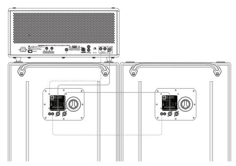
The alternate example shown above is not as common, but is great for daisy-chaining multiple cabinets. You may connect a speaker cable with 1/4" or Speakon ends from one speaker output of the amplifier to the speaker input of the Ampeg SVT-610HLF cabinet. An additional cabinet may be connected by attaching another speaker cable from an open jack (thru) to the input jack of the next cabinet. Multiple cabinets may be daisy-chained this way.
