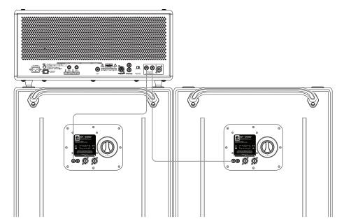
In the example above, a speaker cable with 1/4" ends connects from one speaker output of the amplifier to the speaker input of the Ampeg SVT-610HLF cabinet. An additional cabinet may be connected by attaching another speaker cable from the remaining 1/4" speaker output of the amplifier to a speaker input of the next cabinet.
