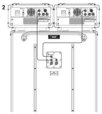
In the "Split (dual)" example **2** above, a speaker cable with 1/4" ends connects from the speaker output of the amplifier to the Upper 4x10 Dual Mode 1/4" input of the Ampeg Heritage SVT-810E cabinet. An additional speaker cable with 1/4" ends connects from the speaker output of another amplifier to the Lower 4x10 Dual Mode/Mono Mode 1/4" input. This configuration allows two amplifiers to separately drive each 4x10 section of the full cabinet.
