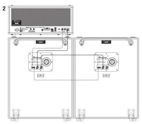
Example 2 above is not as common, but is great for daisy-chaining multiple cabinets. You may connect a speaker cable with 1/4" or Speakon ends from one speaker output of the amplifier to the speaker input of the Ampeg Heritage SVT-410HLF cabinet. An additional cabinet may be connected by attaching another speaker cable from an open jack (thru) to the input jack of the next cabinet. Multiple cabinets may be daisy-chained this way.
