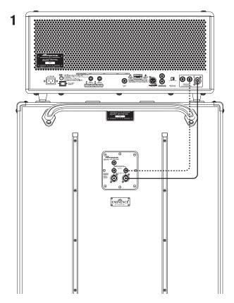
In the "Combined (mono)" example **1** above, a speaker cable with 1/4" or Speakon ends connects from the speaker output of the amplifier to one of the Lower 4x10 Dual Mode/Mono Mode speaker inputs of the Ampeg Heritage SVT-810E cabinet. This configuration allows an amplifier to drive all 8x10 speakers.
