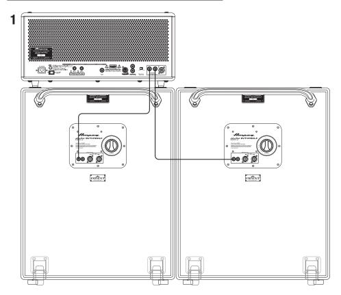
In example 1 above, a speaker cable with 1/4" ends connects from one speaker output of the amplifier to the speaker input of the Ampeg Heritage SVT-410HLF cabinet. An additional cabinet may be connected by attaching another speaker cable from the remaining 1/4" speaker output of the amplifier to a speaker input of the next cabinet.
