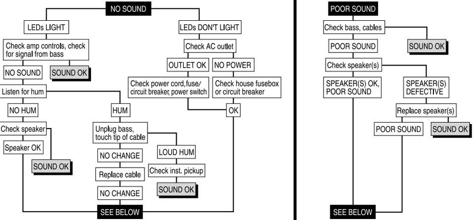
If the problem isn't covered above, or if the steps lead you here, then contact your Ampeg dealer for service information. Also, you should refer the amp for servicing if it gets dropped, has liquid spilled into it, or sustains damage to its power cord.
