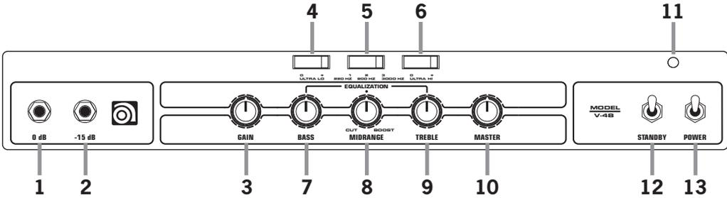
**11. STANDBY/POWER LED:** This is a multi-function LED. In Standby mode, it glows red and in the On mode it glows green.
