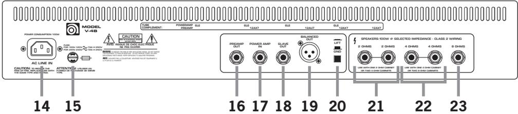
**14. AC LINE IN:** This is where you connect the supplied AC power cord. Plug the male end of the cord into a grounded AC outlet.
