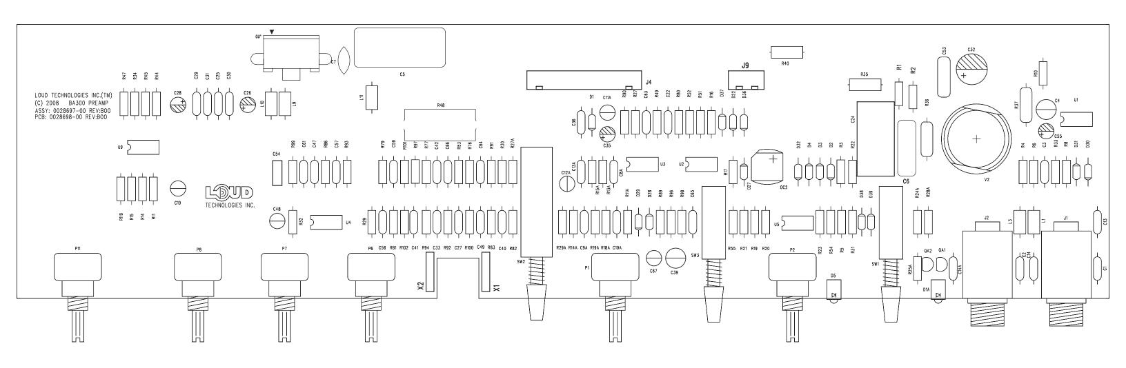
OVERALL FINISH THICKNESS: 1.6mm +/-.125mm DOUBLE SIDE PCB
